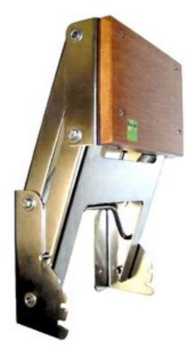
New Zealand's most popular outboard motor mounting bracket for over 36 years. Superior construction means that it is possible to have a motor mounted on this bracket while towing your boat on the road. No parts to come loose or fall off due to use of pressed stainless steel pivots and shake-proof fasteners.
