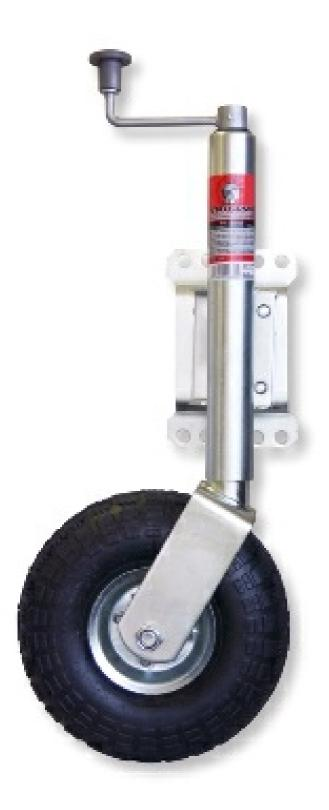
Trojan Pneumatic Premium Jockey Wheel are fitted with a multi fit swivel bracket which can either be bolted to drawbar or fitted using U Bolts.Â
