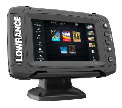
Sporting a five-inch, high-resolution touchscreen display, the Elite-5 Ti has your sonar needs covered with StructureScan® HD compatibility and support for Low/Mid/High CHIRP and 83/200 /455/800kHz frequencies. It has a built-in GPS antenna and trusted Lowrance navigation features, allowing you to navigate with ease.
