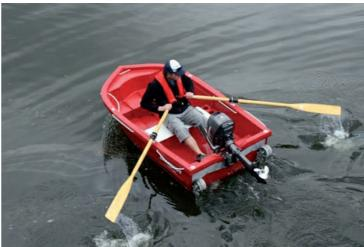
The SW2400 Dinghy is constructed from twin skinned polyethylene and foam filled and is virtually un-sinkable, indestructible and maintenance free. PRICE EXCLUDES FREIGHT FROM AUCKLAND
