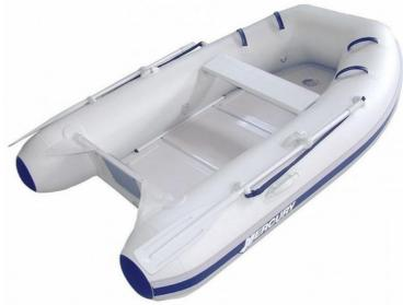
A versatile Boat that can carry up to three Adults and one Child and weighs only 51kg. Featuring thermo-welded seams and fittings and a fiber glass seat. Fantastic wee run about inflatable.
