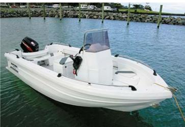
The SW3500 Center Console E-Fish is constructed from twin skinned polyethylene and foam so you can be assured it's virtually un-sinkable, indestructible and maintenance free. Excellent boat for, fishing, rowing clubs, water sports or duck shooting.
